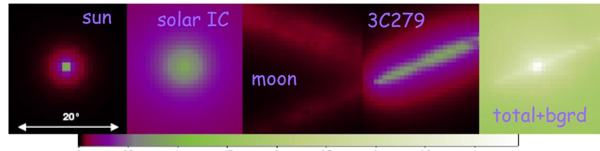
FIGURE 2. Fitted model counts of the main components centered on the Sun. From left to right: Sun disk, Sun IC, moon, 3C 279, and the total predicted counts including uniform background. The colors show the counts/pixel, for  $0.5^\circ \times 0.5^\circ$  pixels.
