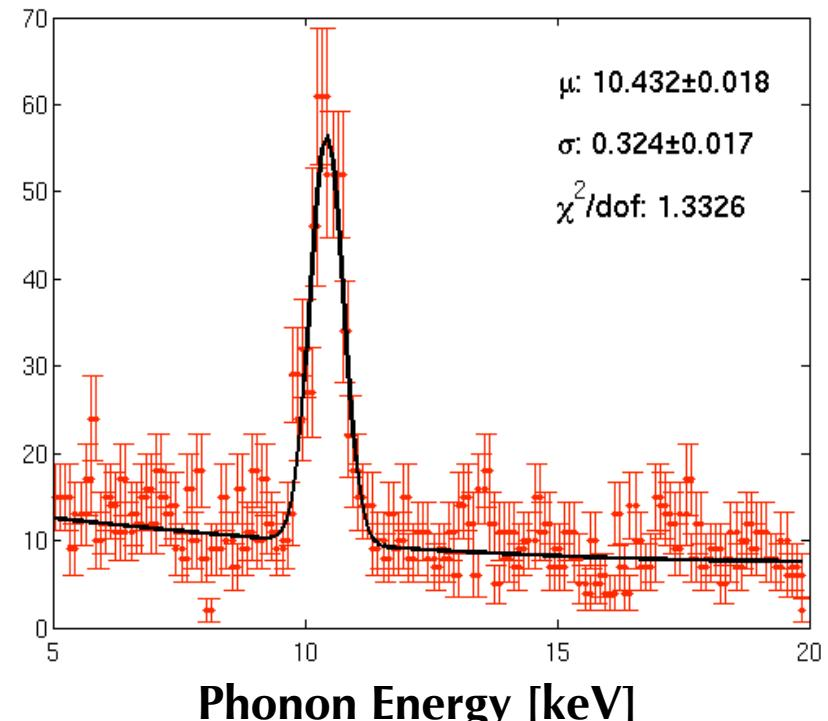
Neutron capture into  $^{70}\text{Ge}$  during the Cf calibration
