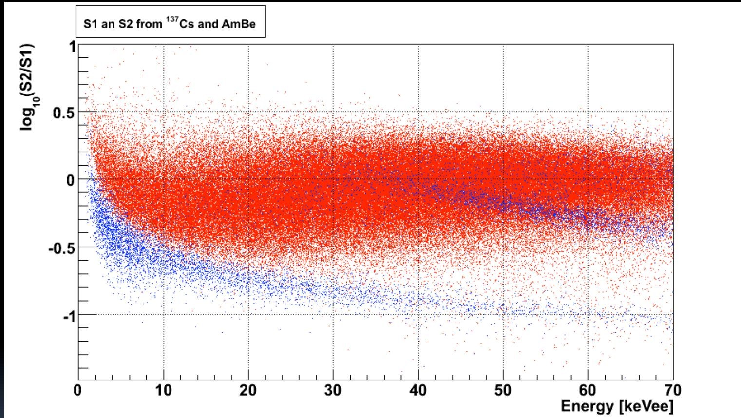
Combined data from runs with  $^{137}\text{Cs}$  (red) and AmBe (blue) sources. Separation of NR and ER bands is very clear. 40 keV line from neutron inelastic scattering is clearly visible on the ER band.
