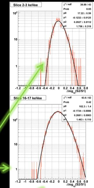
Slicing with 1 keV bin and fitting with skew-normal function:
