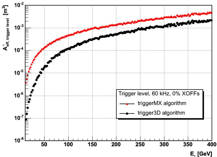
Effective Area at the trigger level, for the default & **directional** trigger algorithm
