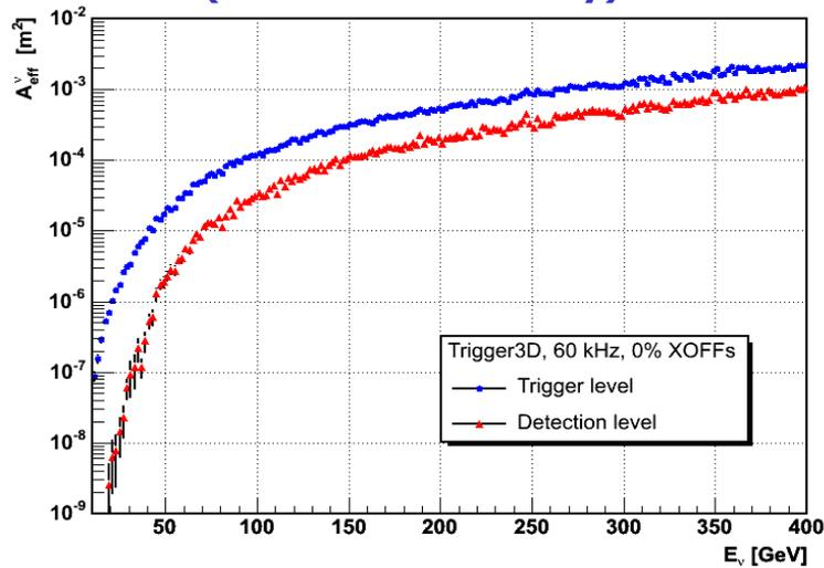
$$\frac{dN_{\text{observed}}}{dt} = \iint A_{\text{eff}}^{\nu}(E_{\nu}, \Omega) \frac{d\Phi(E_{\nu}, \Omega)}{dE_{\nu} d\Omega} dE_{\nu} d\Omega$$
